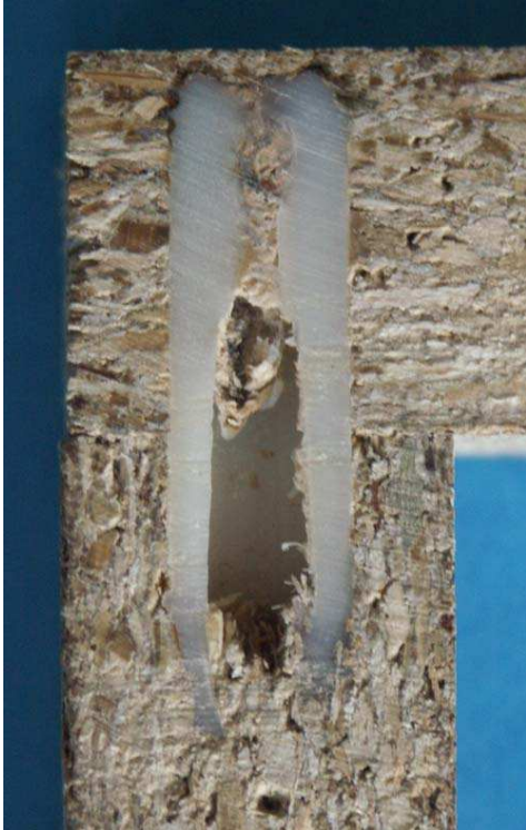
Titusonic ® Cabinet Assembly – Detail of Corner Fixation
