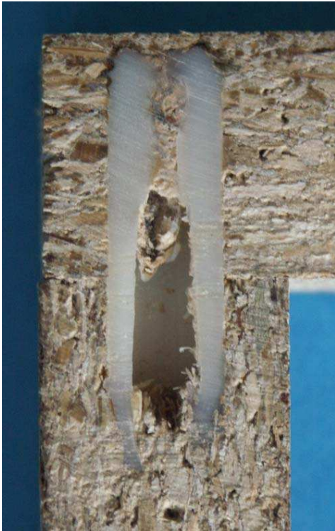
Titusonic ® Cabinet Assembly – Detail of Corner Fixation
